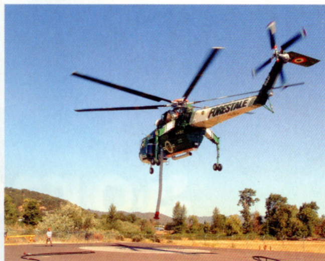
The Sikorsky S-64 is a hugely capable machine whether slinging a grapple full of logs or dropping retardant on a wildland fire (opposite page). One of the cranes built for the Corpo Forestale dello Stato, the Italian State Forestry Corps (far left). A pond snorkle dangles below the ship—it allows the 2,650-gallon tank to refill from hover in 45 seconds.
